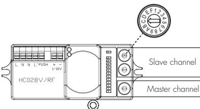
Both slave and master can be set to 16 different channels (Hexadecimal setting).
