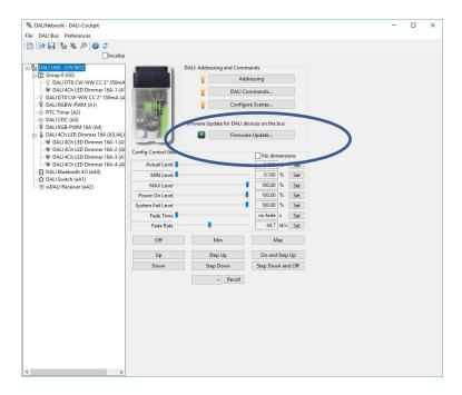
Then press the "Firmware Update" button and enter the activation key to enable this tool. Select the device and the location of the software and press Start.
