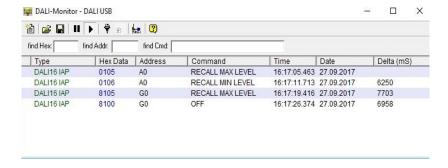
The monitor log can be saved to a file. This can be an important help for various analysis.
