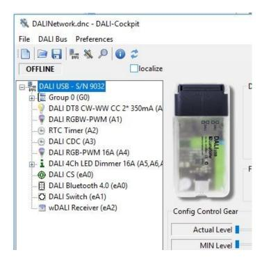
When OFFLINE appears above the component tree the devices can be accessed without loading data from the bus.
