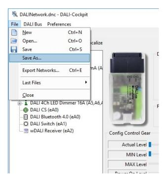
After the file is saved, it can be opened without connection to the DALI line. To look into the configuration of the devices, Offline Mode has to be activated (DALI Bus  $\rightarrow$  Work Offline).
