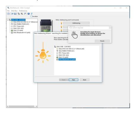
In this example we will add a DALI switch and a wDALI Remote. When detected correctly the components will be added in the DALI device list as shown below.
