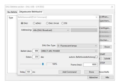
For each command in the list a destination address and the DALI command can be configured. Furthermore the delay time after the command can be defined. E.g. adding 3 Direct Act Power Cmds for different destinations to the command list will result in a list like the following:
