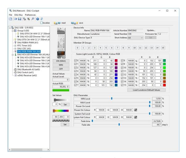
DALI controls configuration sites are divided in a device info block and a device setting block. The device setting block often consists of several tabs, in most cases a general settings tab and a tab for each input or sensor (depending on device).
