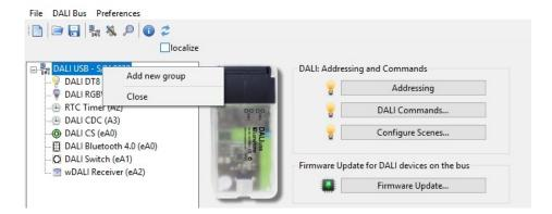
For adding group members just use the drag and drop function in the component tree. Groups are always displayed at the top of the component tree, below all addressed devices are listed. Selecting the group window allows to send configuration and control commands to the according group.
