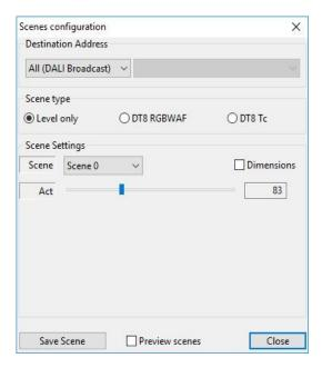
In the menu you can enter the effective range you want to configure, the type of scene (level only or special DT8 color scene type), the scene number and the values. Pressing "Save Scene" will store the parameters to the devices affected by the selected address range.
