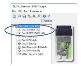
Sometimes it can happen that a DALI Conflict is shown in DALI Cockpit, if you add additional devices to an existing DALI system. To resolve this, delete this DALI address and do a new addressing procedure (extension).
